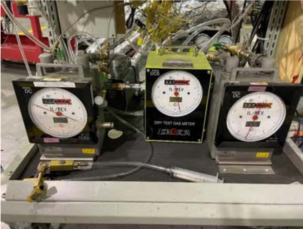
Picture 11: Dry gas meter
